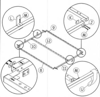
Join together all the bed base parts (8),(9),(10),(11) and (12) using hardware parts **M**. Attach hardware parts **L** using hardware part **M** and than attach hardware part **U** by slot to the part (11) as shown. **Important note: Please assemble follow arrow direction.**
