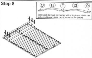
Place wood slats with plastic caps as above drawing. Then, fix it on the bed base by pressing it accordingly to the default holes. Ensure the plastic cap's pin is aimed to the hole.
