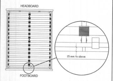
Adjust the bed base, make sure distance with the front footboard approximately 15mm to above gap as shown.
