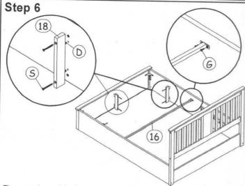
Fix support wood to the side rails and footboard with hardware as shown and follow by centre cross bar.
