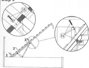
Assemble the bed base on the right & left hydraulic frame and fix bolts starting from '1' to '3' as shown.
